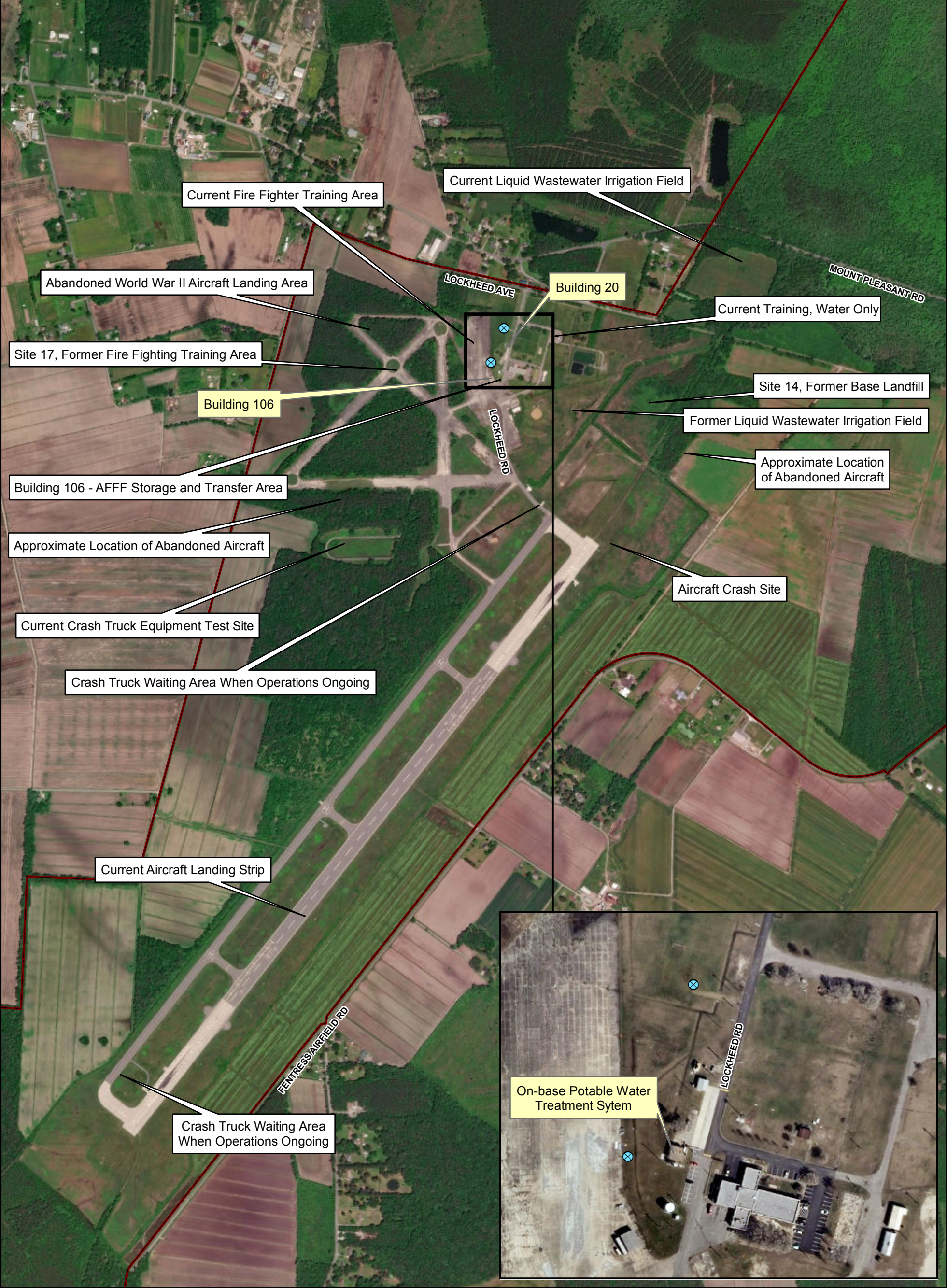
Figure 2-2 Potential PFAS Source Areas and On-base Potable Water Treatment System Engineering Evaluation and Cost Analysis for Drinking Water NALF Fentress, Chesapeake, Virginia
