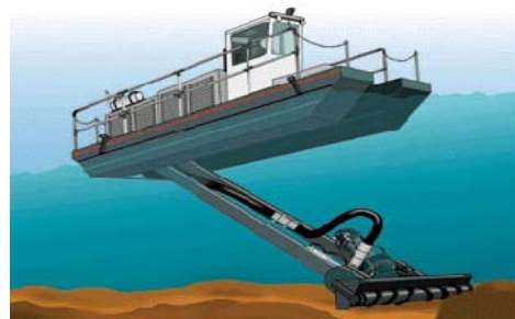
Hydraulic dredging techniques will be used to remove sediments from the Pier 1 Inner Area
